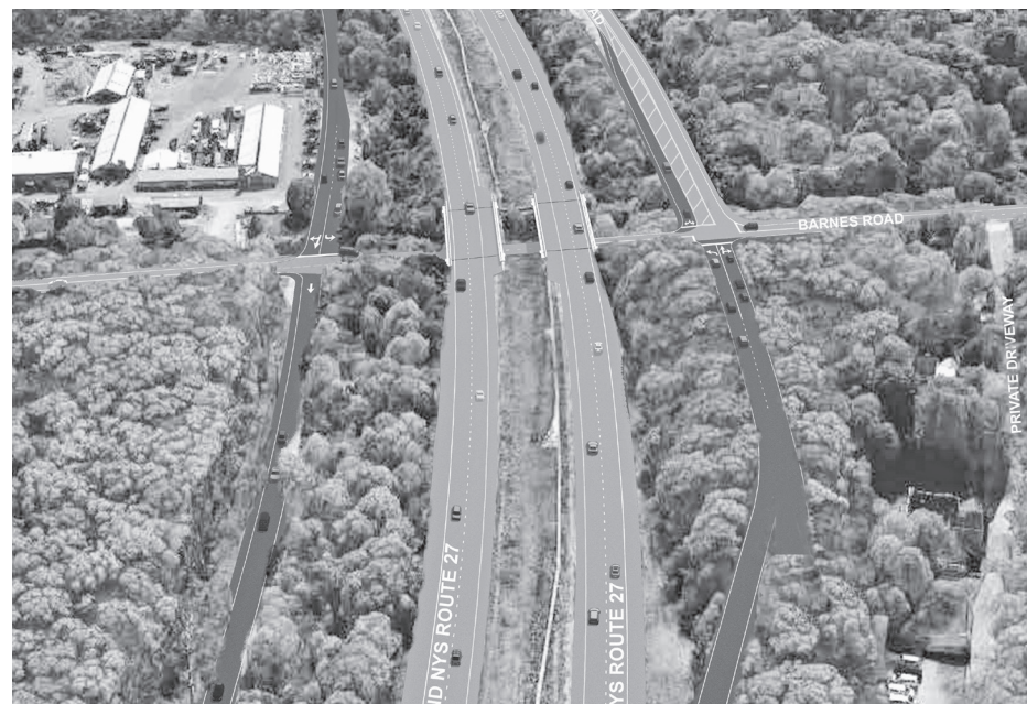
A rendering of the Barnes Road interchange project shows a new exit connecting the street with Sunrise Highway on the north and south sides.
